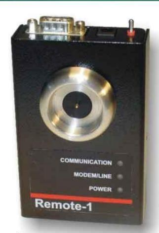
Physical characteristics: Body in aluminum with epoxy painting
