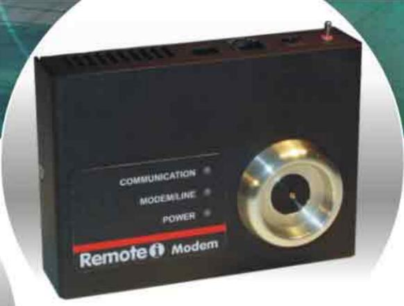
**Remote-i** is available in two versions, MODEM or STANDARD, both very easy to use. The MODEM version is connected to a power source and a phone line. It comes with its own internal modem of 14400 bps and is always ready for use. The STANDARD version requires an external modem in order to carry out the transmissions. Contronics recommends for the STANDARD version the US Robotics 56k, not included.
